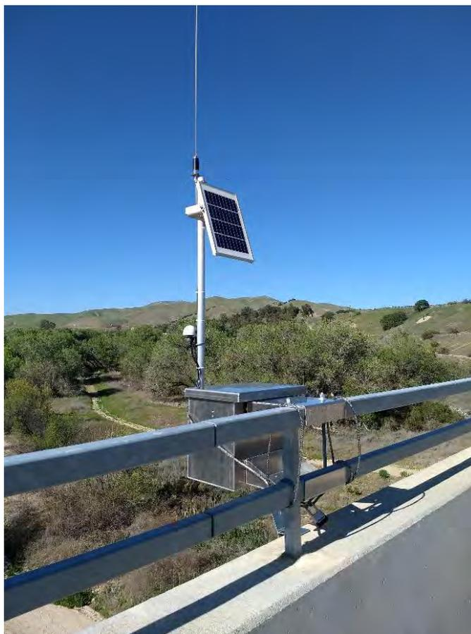
*Figure 3. San Miguel (Salinas River) radar sensor stream gage installation*
